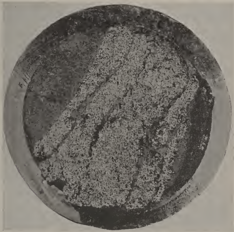
FIG. 241.—View of area of rupture of bolt that failed due to repeated stress, showing evidence of progressive failure. (Obtained by Prof. H. F. Moore).
